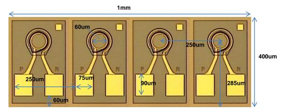
Attention: GaAs material and electrostatic sensitive device, observe precaution for handling.
